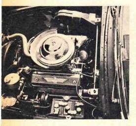
The big, 292-cubic-inch engine (same as Mercury displacement) develops 198 horsepower and gives the Thunderbird performance that is spectacular.
